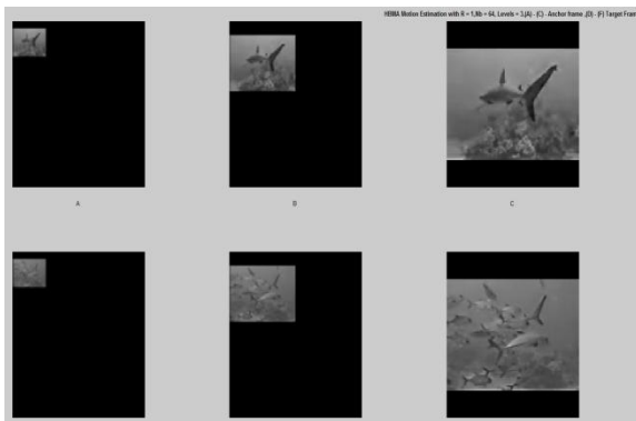
Figure 21: HBMA for shark.avi when No of blocks=64
